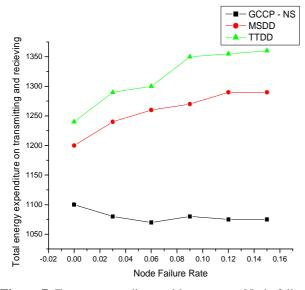
Figure 7. Energy expenditure with respect to Node failure rate
