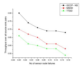
Figure 5. Throughput with respect to sensor node failures
