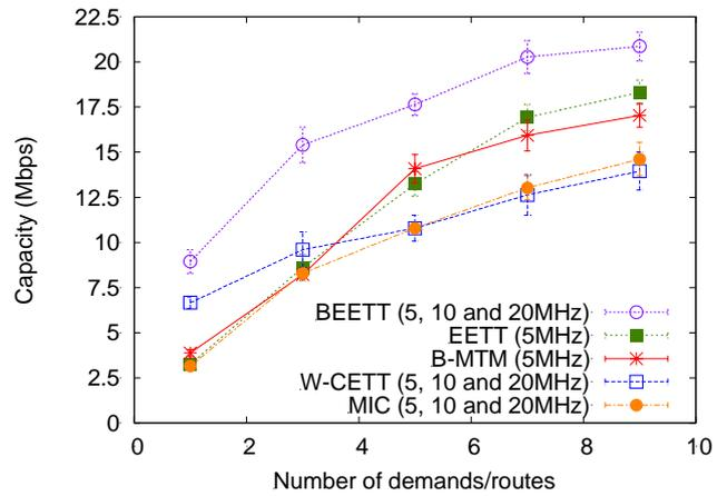
Figure 20. Greater obtained capacity values by selecting or using individual channel widths of 5, 10 and 20MHz)
