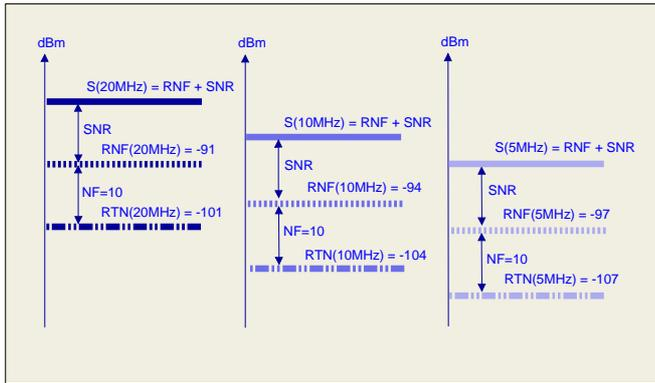
**Figure 6.** Minimum receiver sensitivities for channel widths of 5, 10 and 20MHz
