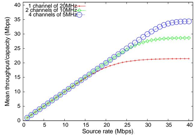
**Figure 5.** Throughput and capacity of 1, 2 and 4 orthogonal channels of 20, 10 and 5MHz. (Exponential source)
