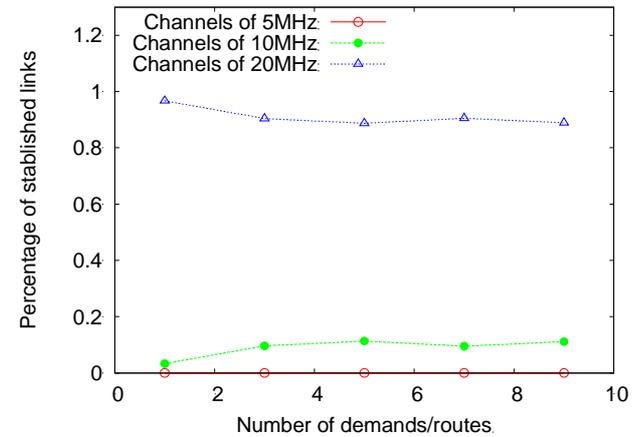
Figure 10. Percentage of established links in each channel width for WCETT metric
