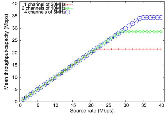
**Figure 4.** Throughput and capacity of 1, 2 and 4 orthogonal channels of 20, 10 and 5MHz. (CBR source)
