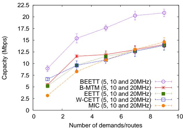
Figure 19. Obtained capacity when selecting among existing channel widths (5, 10 and 20MHz)
