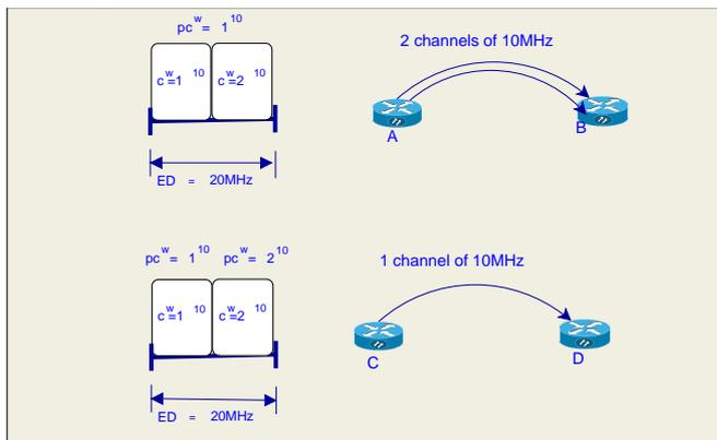
**Figure 2.** Spectrum division into physical (group of channels) and individual channels
