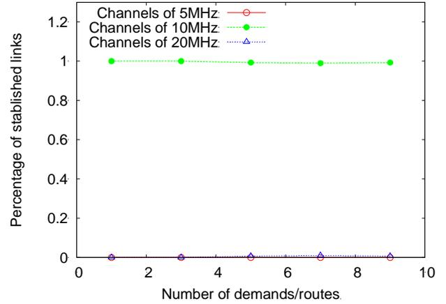
Figure 14. Percentage of established links while selecting channel width for B-MTM metric
