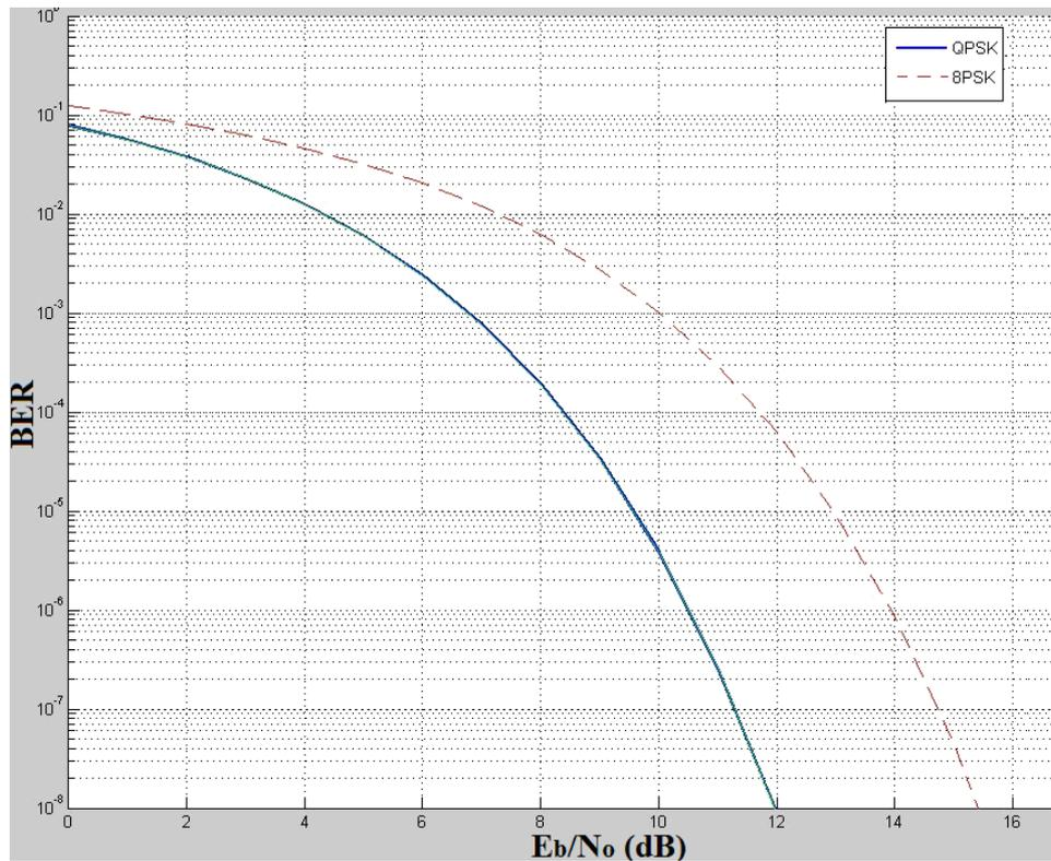
Fig.16: Waterfall curves for the QPSK and 8PSK
