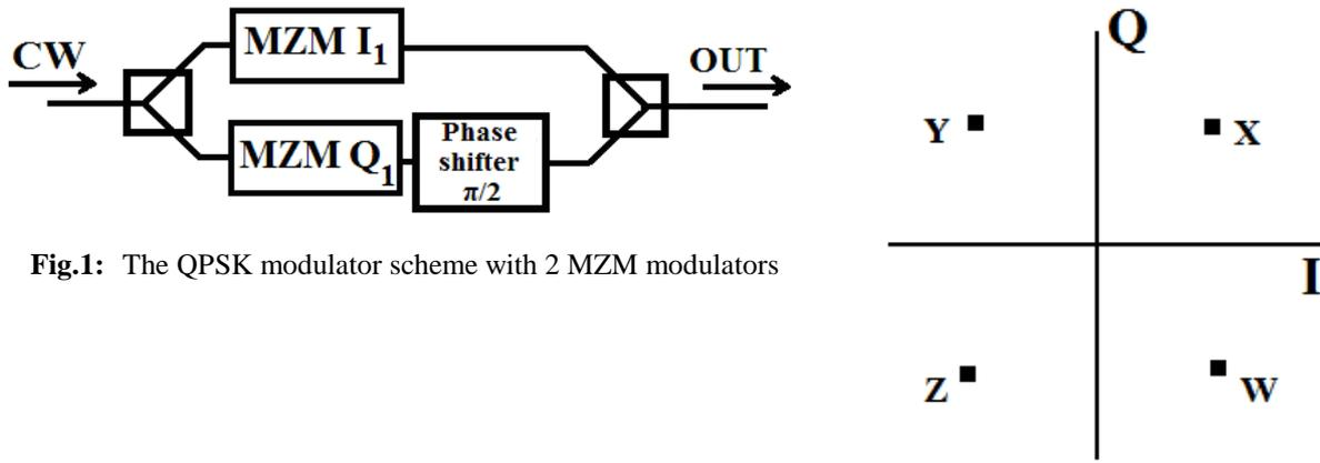
Fig.1: The QPSK modulator scheme with 2 MZM modulators
