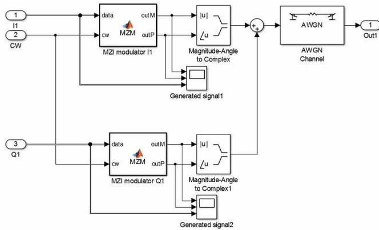
**Fig.10:** The QPSK 1 modulator block scheme
