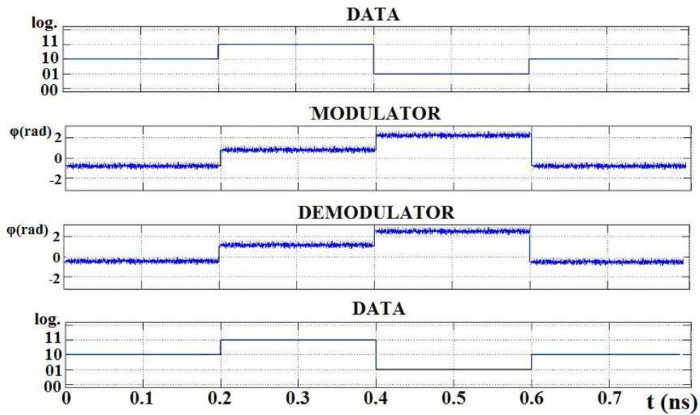
Fig.15: QPSK optical signals
