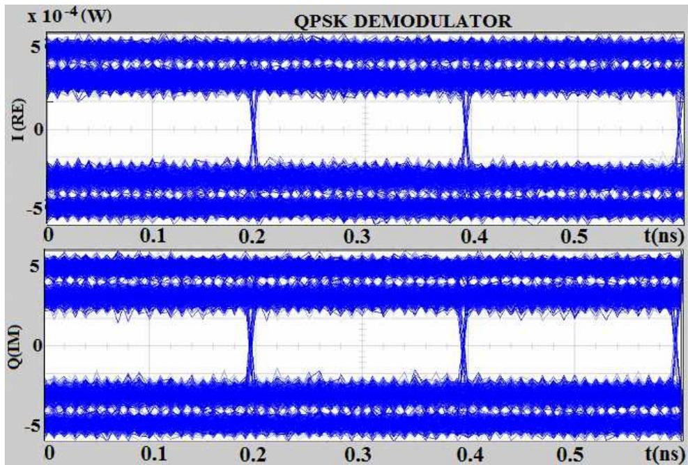
Fig.18: The QPSK eye diagram
