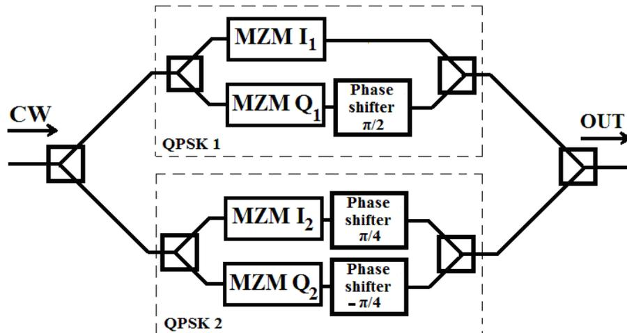
Fig.3: The 8PSK modulator scheme with 4 MZM modulators
