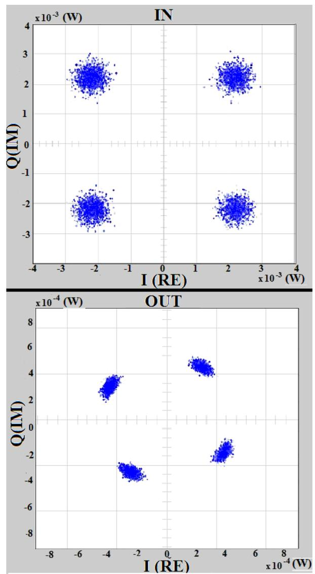
Fig.13: QPSK constellation diagrams
