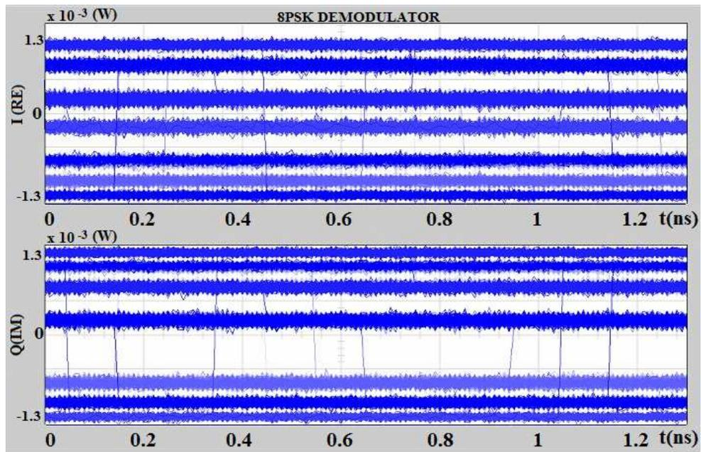
Fig.17: The 8PSK eye diagram
