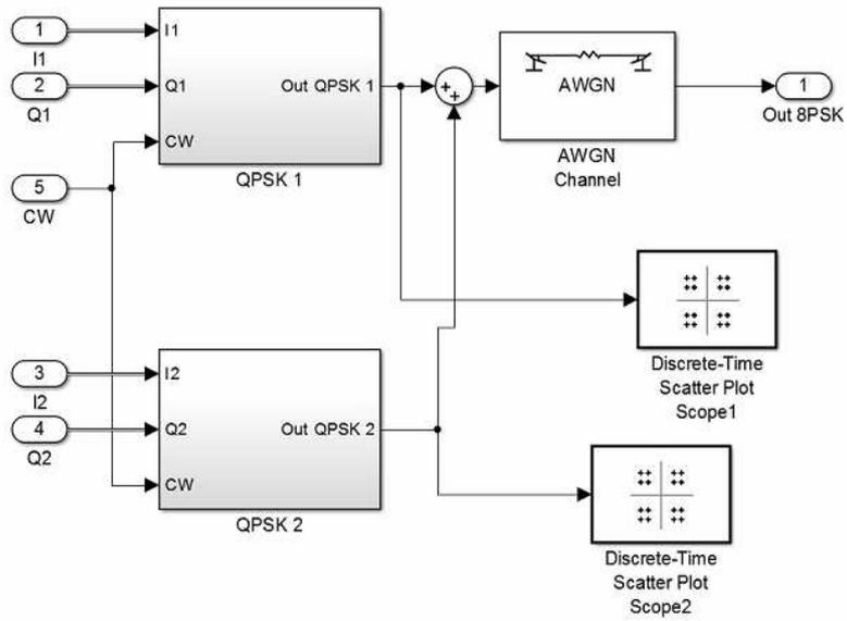
**Fig.9:** The 8PSK modulator block scheme
