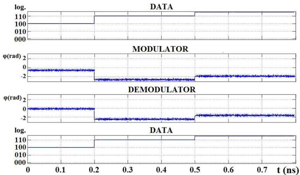
Fig.14: 8PSK optical signals
