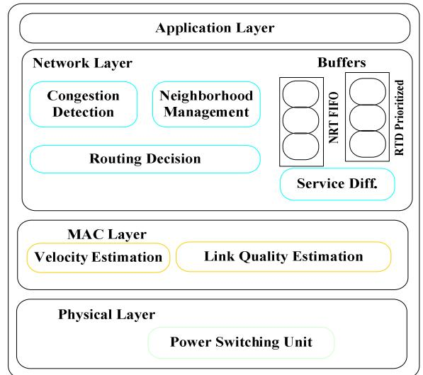
**Figure 1.** Proposed Cross layer architecture
