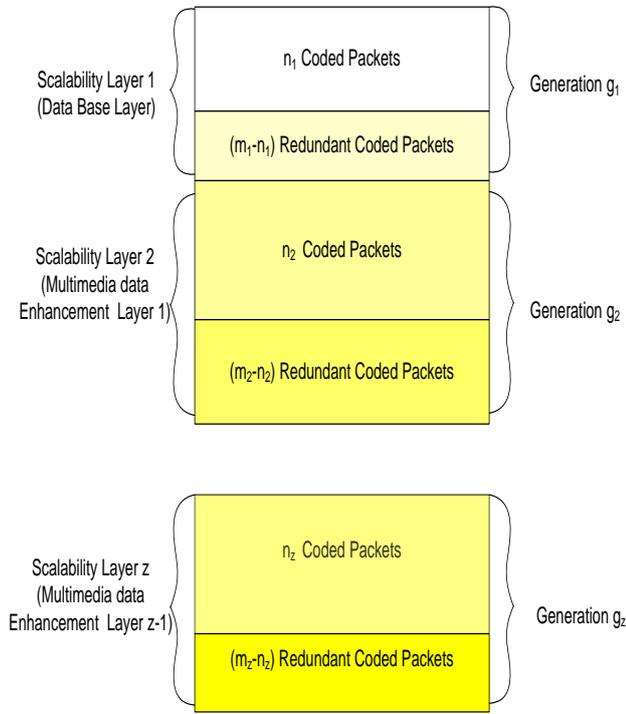
**Figure 3.** Multimedia data packet assignment to S-RLNC generations in MGM approach
