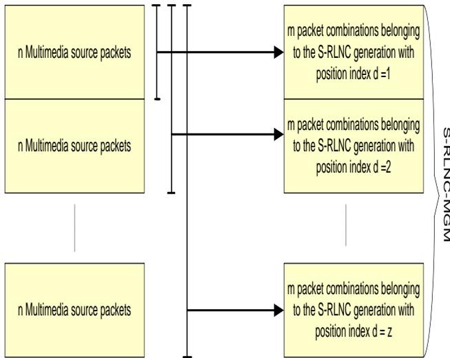
**Figure 2.** S-RLNC with multi-generation mixing (MGM)
