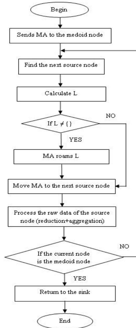
**Figure 7.** Flowchart of the communication process of mobile agents
