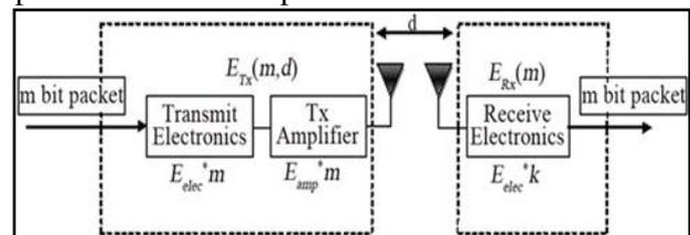
**Figure 1.** Energy consumption model in wireless sensor networks[15]
