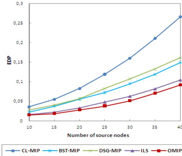
**Figure 10.** Energy-delay product in terms of the number of source nodes in the network
