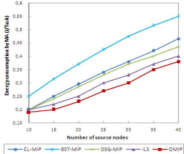
**Figure 8.** Energy consumption by mobile agent in terms of the number of source nodes in the network
