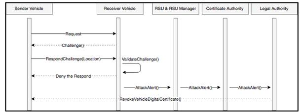
**Figure 4:** Vehicle Communication Sequence Diagrams (Attack Case)
