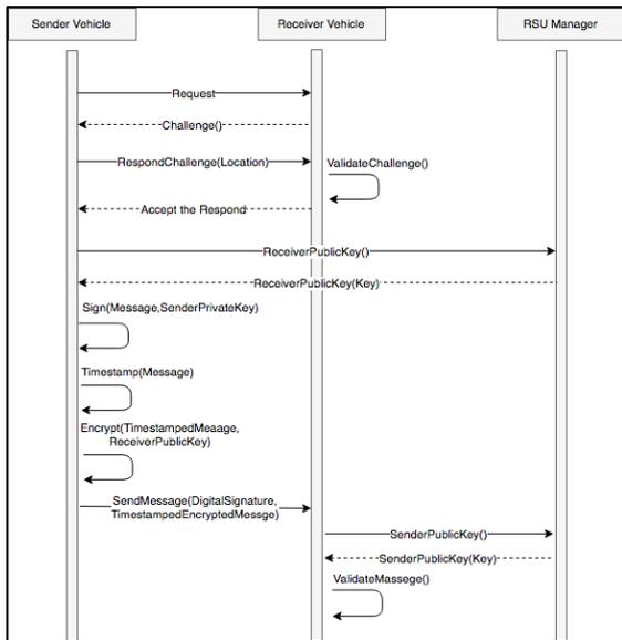
**Figure 3:** Vehicle Communication Sequence Diagrams (Successful Case)
