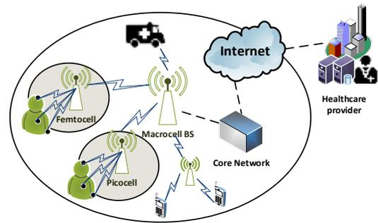
Figure 2. Illustration of multitier heterogeneous networks incorporating medical sensors in 5G communication networks.
