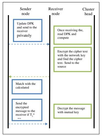
Figure 4. Key Authentication and Verification Phase of the Proposed MSKM Protocol
