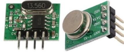
Figure 4. The 433 MHz ASK/FSK transmitter devices
