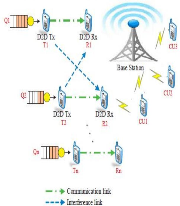
**Figure 2.** Interference in Device to Device communication
