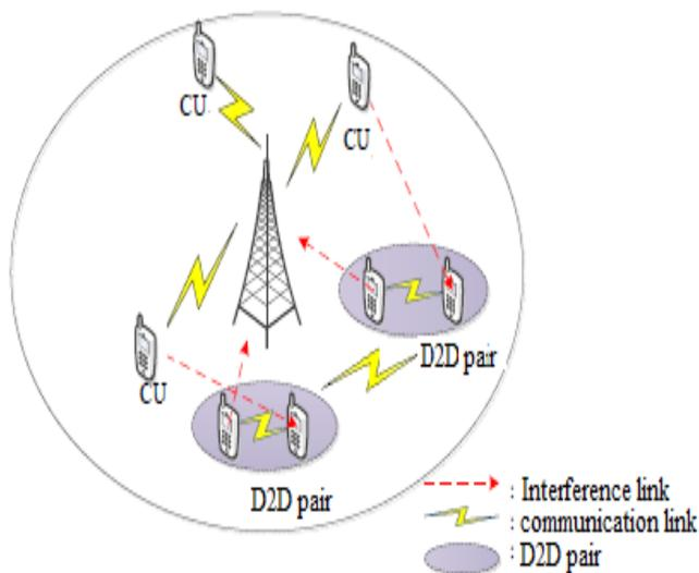
**Figure 1.** A single base station with multiple device to device and cellular users
