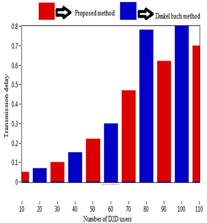
Figure 5. Data transmission delay of D2D users
