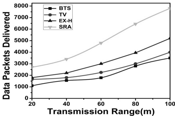
Figure 6(c). Data Packets delivered vs. Transmission Range.
