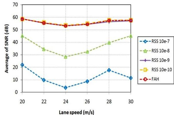
Figure 9. Average of SNR from handover simulation
