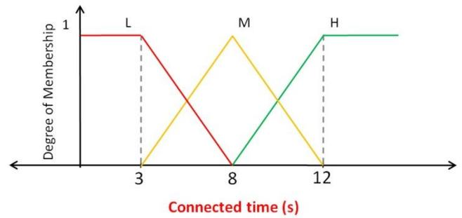
Figure 6. Membership function related to connected time
