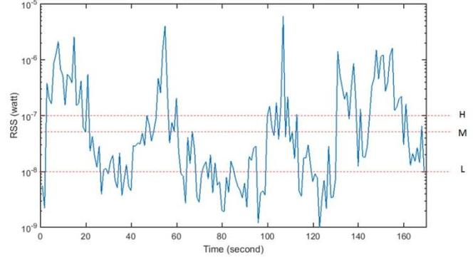
Figure 7. Value range of RSS for estimating the membership function related to RSS
