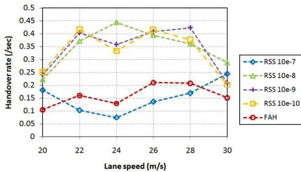
Figure 10. Handover rate from handover simulation
