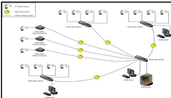
Figure 4. The utilization of FO link in VDS [33].
