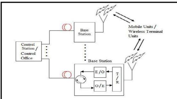
Figure 2. Basic diagram of RoF system [11]
