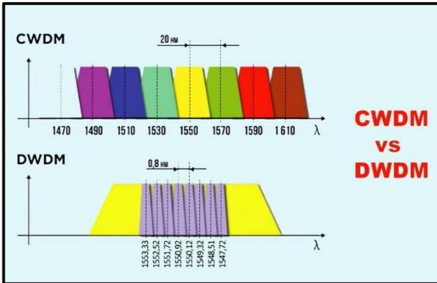
**Figure 11.** The spectrum concept of both CWDM and DWDM [11].
