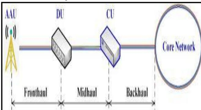
**Figure 13.** The interconnection of front-haul, mid-haul and back-haul[40].
