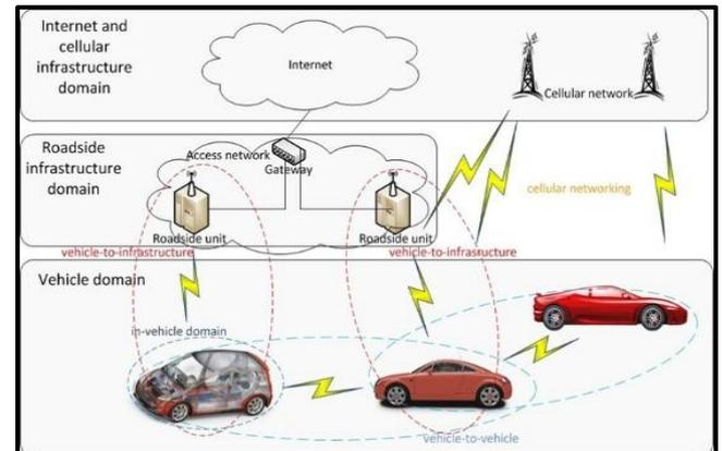
Figure 7. Vehicle communication scenario with RoF system [35].
