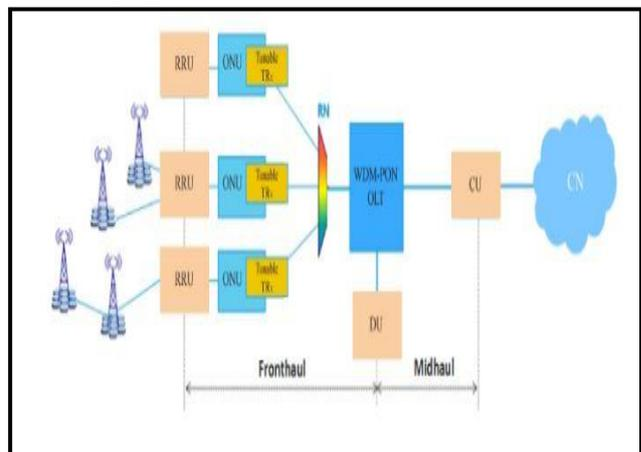
**Figure 14.** The structure of WDM-PON network [42]
