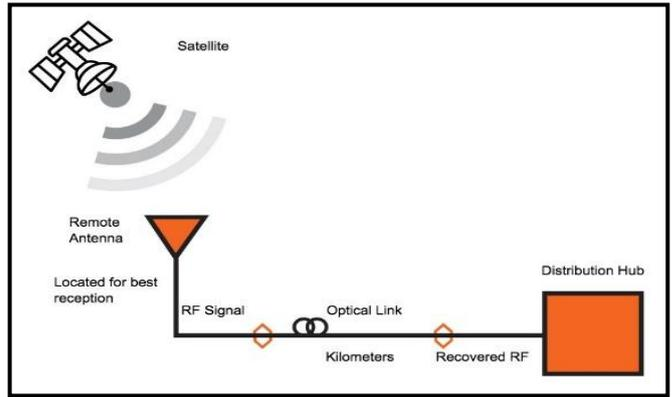
Figure 5. The utilization of RoF for satellite communication [33]
