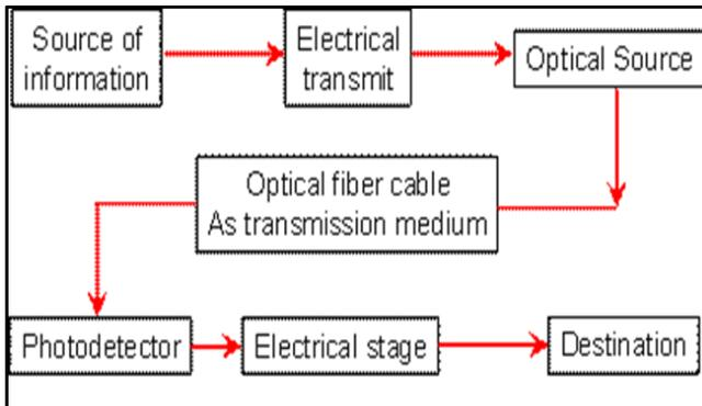
**Figure 1.** Overview on the Basic diagram of FO communication system
