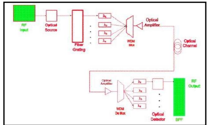
Figure 10. Diagram of RoF system based WDM technique [37].
