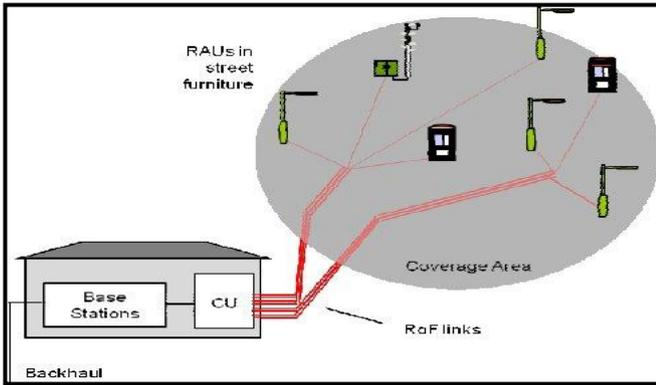
Figure 8. The utilization of RoF in Mobile broadband services [36].
