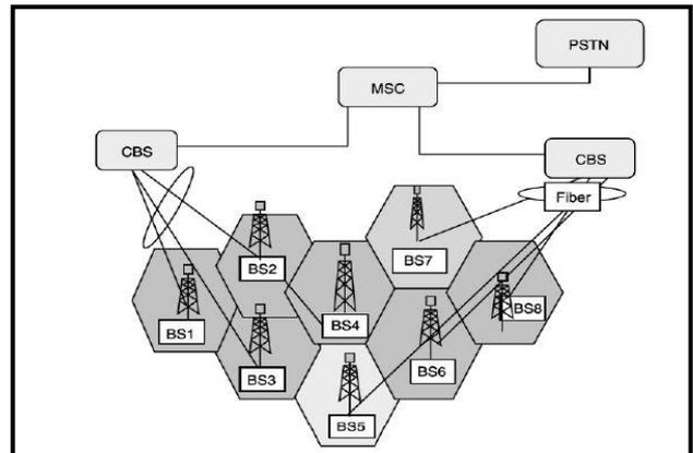
Figure 6. Optical utilization in cellular based network [34]
