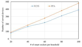
Figure 3: Number of served devices under FCFS and PPA algorithms with different number of sockets per household whilst keeping the maximum power below 10 kW
