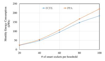
**Figure 2:** Monthly Energy consumption under FCFS and PPA algorithms with different number of sockets per
