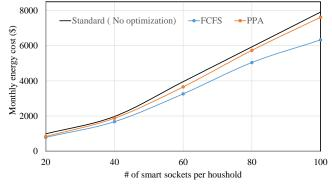
Figure 4: Monthly Energy cost under standard (no-control), FCFS and PPA algorithms with different number of sockets per household
