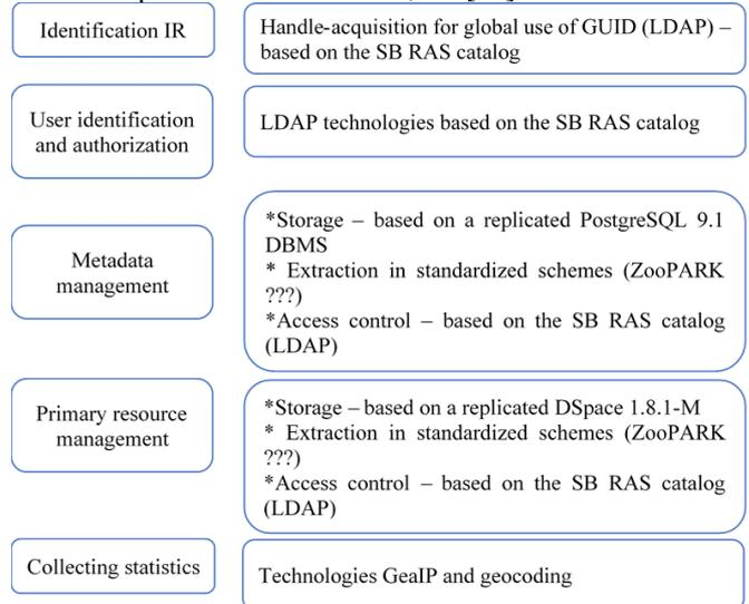
**Figure 3.** Basic technologies of the DIS component
