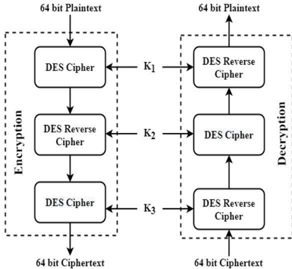
Figure 4. The working of 3DES [8]
