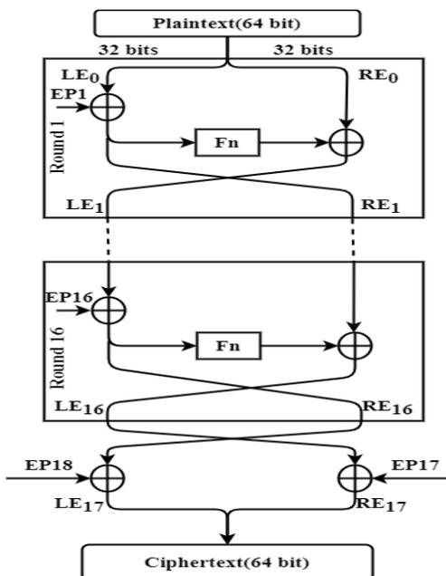
Figure 5. The working of Blowfish [1]
