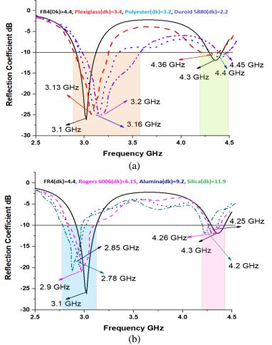
*Figure 10.* Parametric Analysis with Change in Substrate Material, (a) Dk above 4.4, (b) Dk below 4.4
