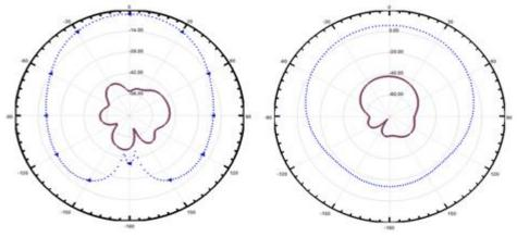
Figure 7. Radiation Pattern in E & H-Field
