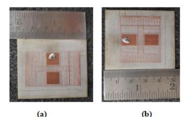
Figure 3. Prototyped Antenna Dimensional View (a) Horizatal view (b) vertical view
