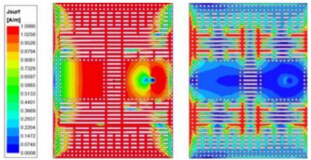
Figure 8. Surface current distribution, (a) 03.10 GHz, (b) 04.30 GHz
