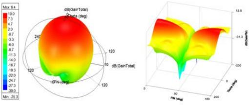
Figure 5. 3D-Gain at 3.1 GHz
