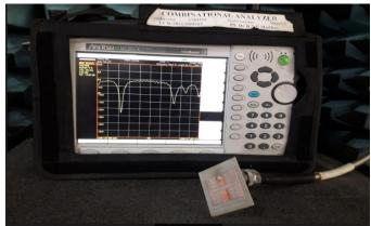
Figure 9. Measurement of S<sub>11</sub> on Anritsu VNA
