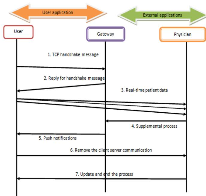
Figure 3 Data transfer process from user to application layer
