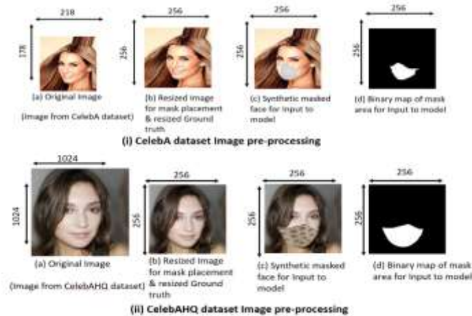
Fig. 4 Preprocessing of the image dataset (data resizing, mask placement & binary map segmentation)
