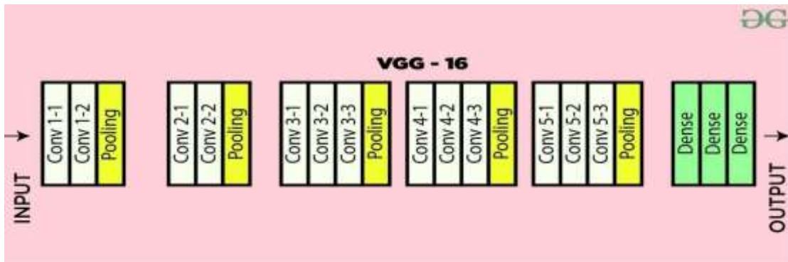
Fig.9. VGG16 layered architecture[20]
