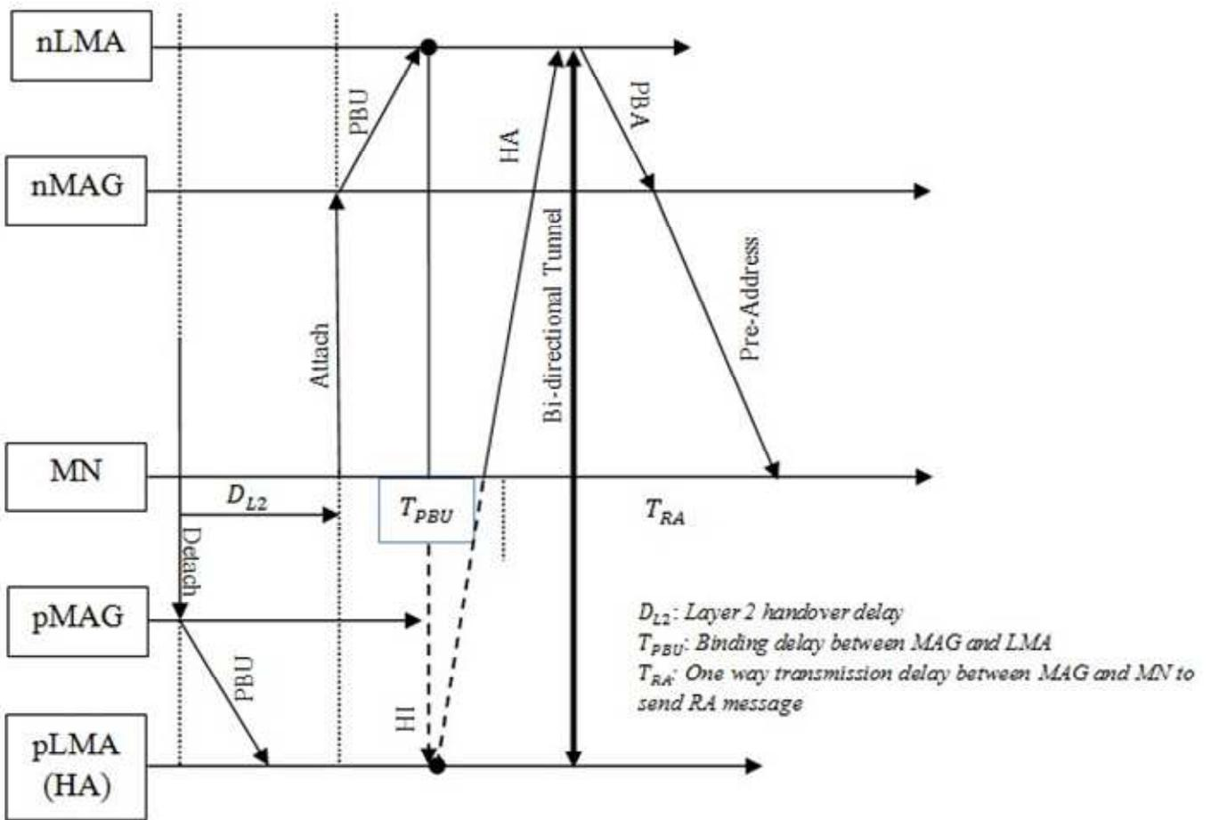
Figure 9. Novel Inter-domain PMIPv6 Handover Procedure and timing diagram
