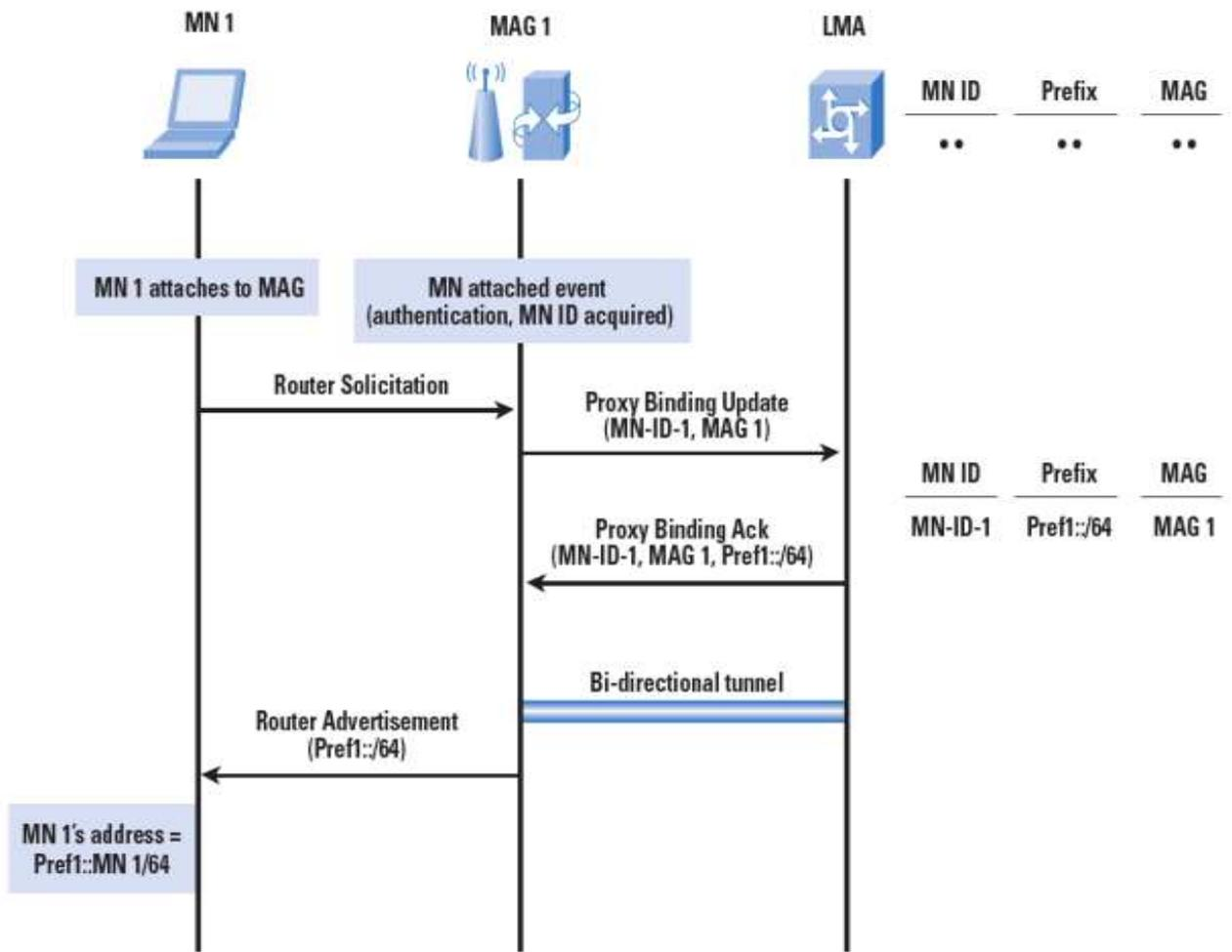
Figure 1. The Procedure of MN Joining a PMIPv6 domain
