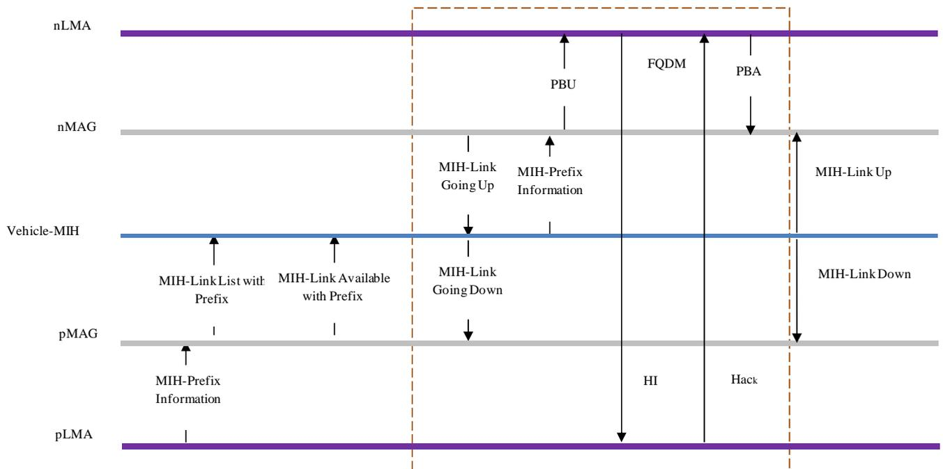
Figure 4. Novel Handover Mechanism Using MIH
