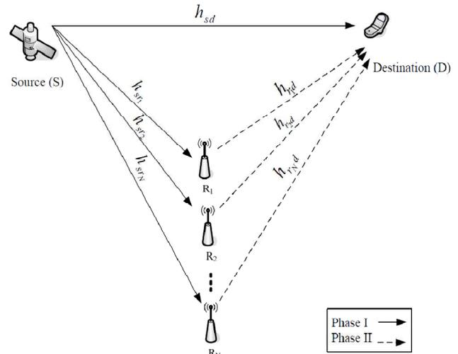
**Figure 1.** An integrated satellite-terrestrial cooperative system
