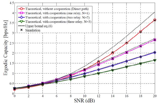
**Figure 2:** Ergodic capacity analysis of the multiple relay integrated satellite-terrestrial cooperative system, the direct channel  $S \rightarrow D$  experience deep shadowing,  $m_0 = 2.56$ , where the  $S \rightarrow R_i$  channel have LOS,  $m_0 = 26$  and the  $R_i \rightarrow D$  channel experience Nakagami-  $m$  fading at  $m = 1$
