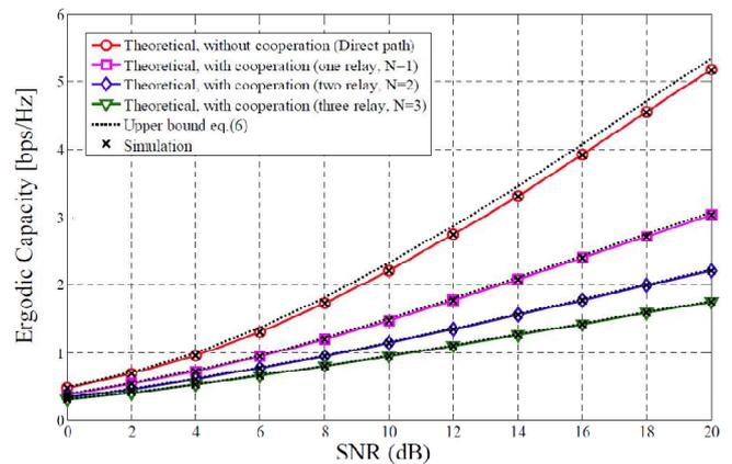
**Figure 5:** Ergodic capacity curves of multiple relay integrated satellite-terrestrial cooperative system, when the satellite channels,  $S \rightarrow D$  and  $S \rightarrow R_i$  experience moderate and light shadowing respectively where the  $R_i \rightarrow D$  link experience Nakagami-2 fading.
