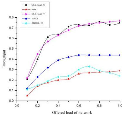
**Figure 5.** The Network Throughput Vs Offered Load
