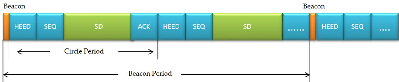
Figure 2. Typical structure of a Beacon Frame
