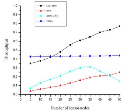
**Figure 6.** The Network Throughput Vs Sensor Nodes
