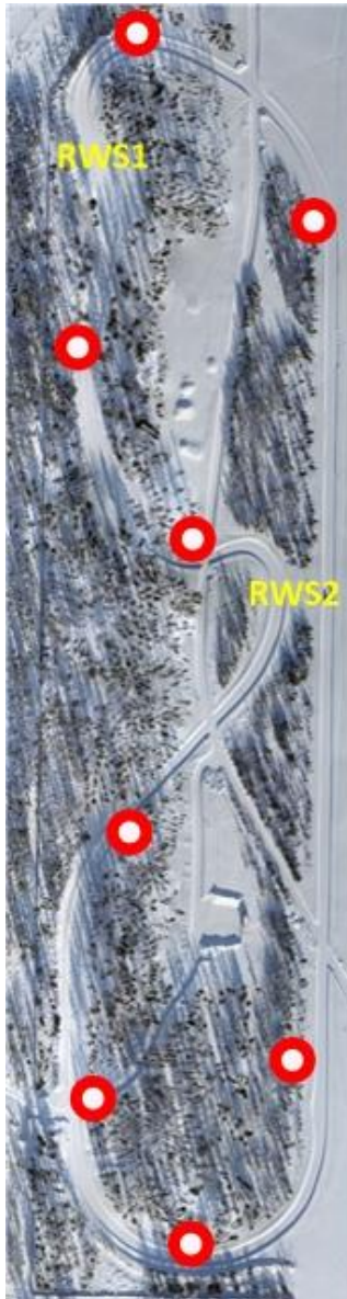
Figure. 1. Sod5G test track. The Road Weather Stations are marked as RWS1 and RWS2, IoT road weather sensors as red circles.
