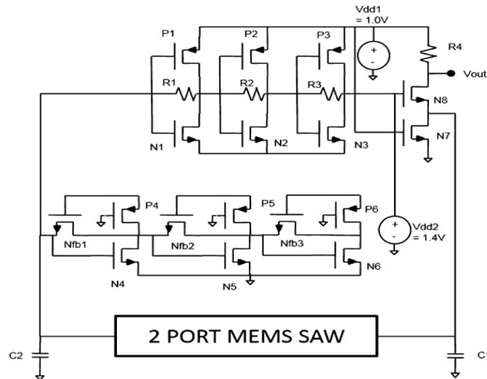
Figure. 10. Boosted Pierce Oscillator Circuit
