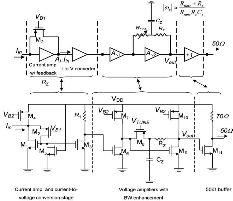
Figure. 7 Diagrammatic Representations of the Tia Showing the Active Pre-Amplification
