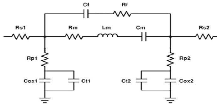
Figure.9. SAW Resonator Circuit
