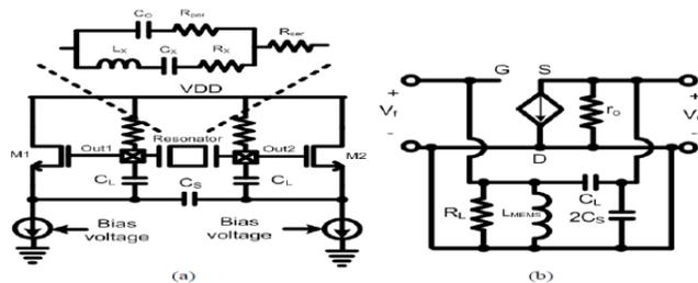
Figure.8 (A) Colpitts Oscillator (B) Its Tiny Signal Model
