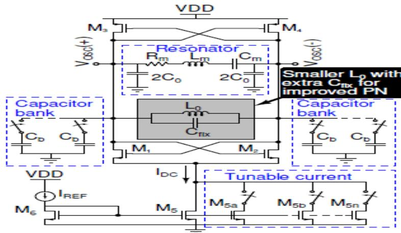
Figure 12 Schematic for A MEMS Resonator on a 30 GHZ Oscillator
