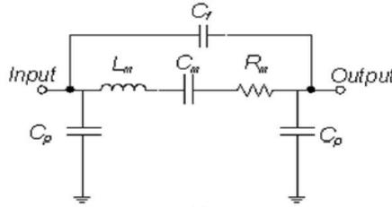
Figure.6 the LBAR's Equivalent Lumped Electrical Model
