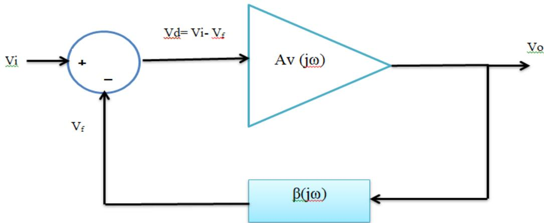
Figure. 2 Block Schematic of the Feedback System
