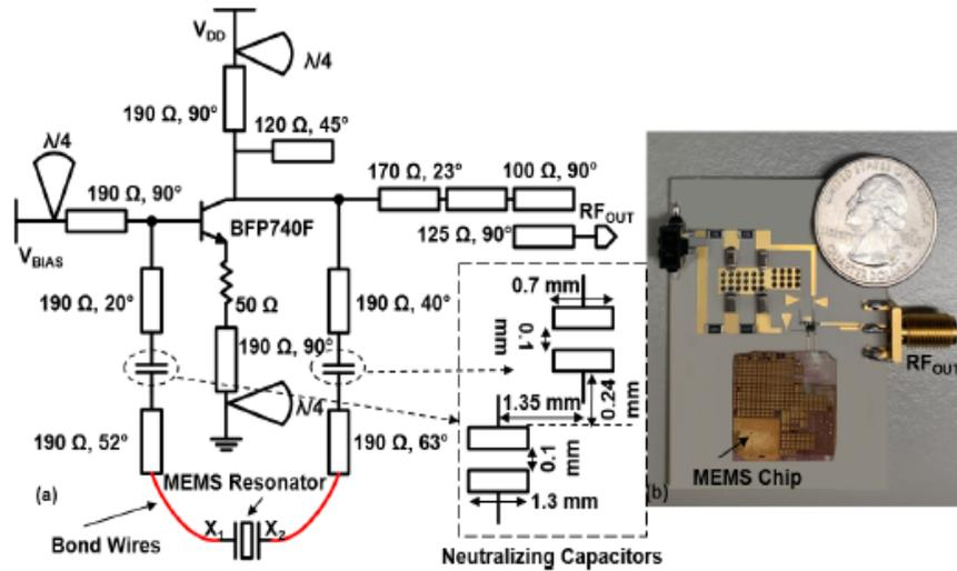
Figure 11. (A) the RF Section of the 13-GHz Oscillator in A Simplified Design. (B) Oscillator PCB.
