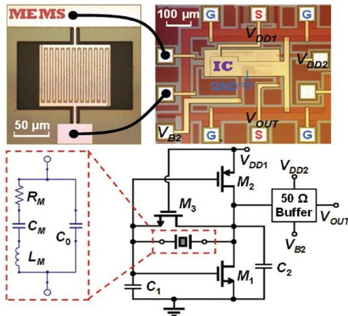
Figure. 5. CMOS IC Chip Wire-Bonding and the MEMS Resonator's Micrographs and Circuit Diagrams
