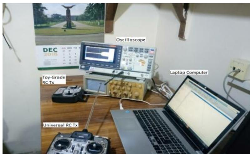
Figure 5. Experimental Setup in an Office Environment
