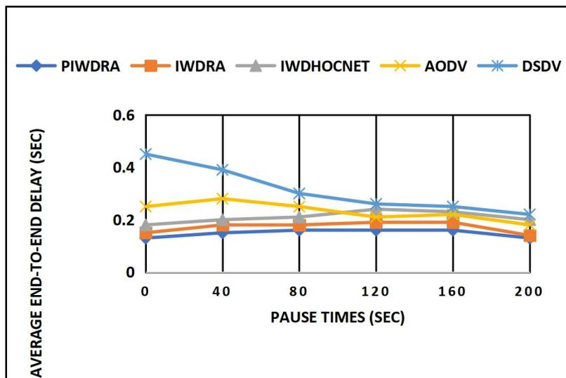
Figure 4. Average End-to-End Delay Under Various Pause Times
