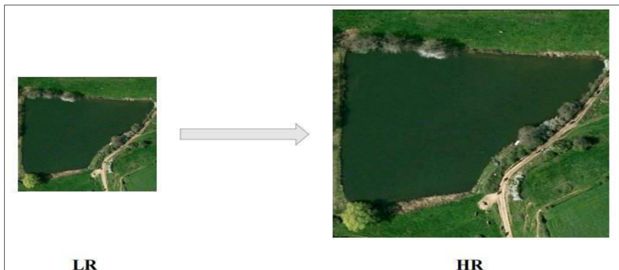
Figure 1. SR aims to reconstruct a high-resolution (HR) image from its degraded low-resolution (LR) counterpart.
