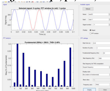
Figure 19 . THD for 33 level inverter
