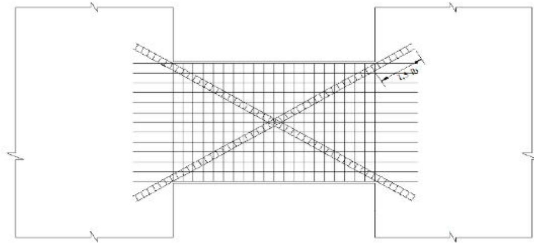
Fig 2. Coupling beam of shear wall
