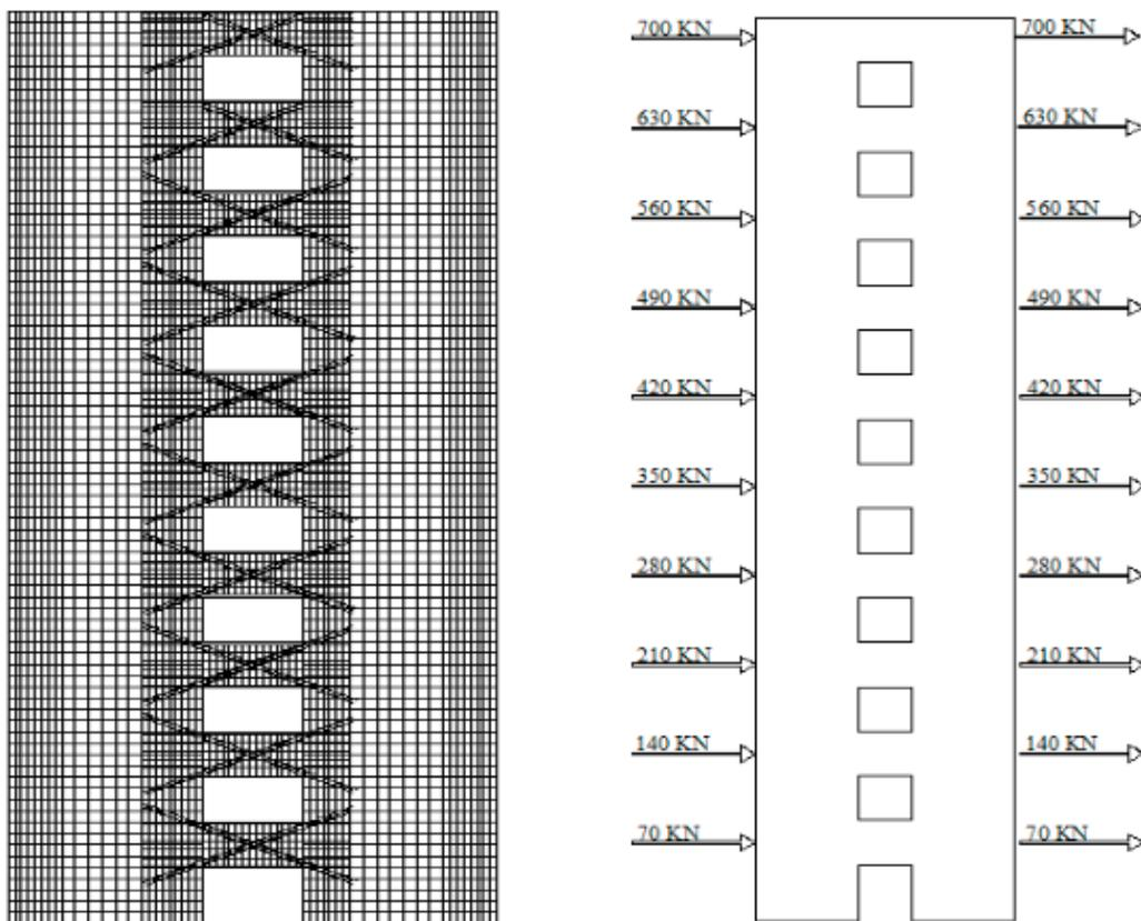
Fig 3. Geometry of coupled shear wall and lateral forces imposed on the structure
