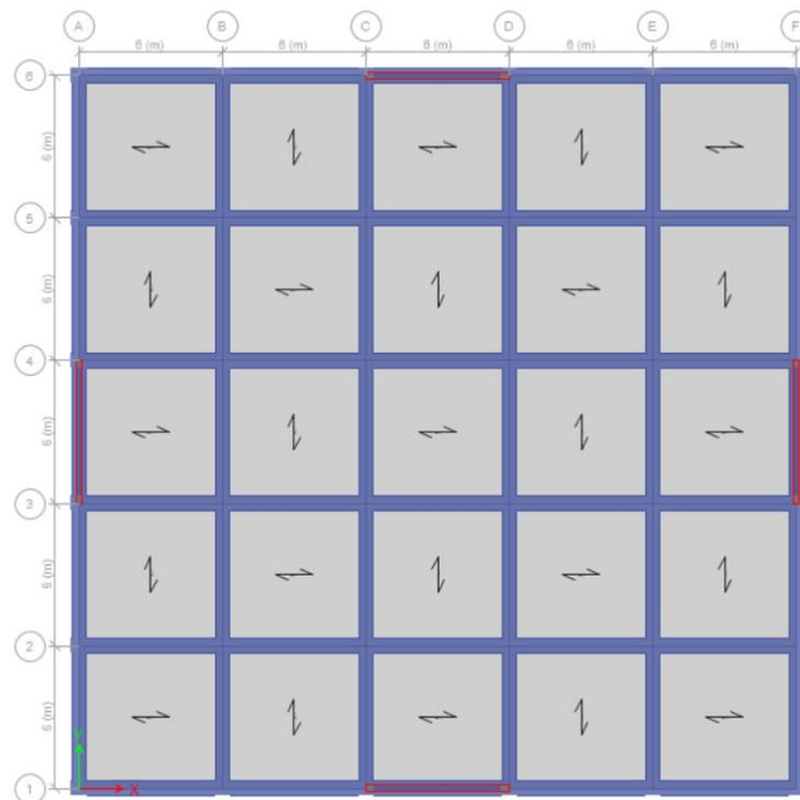
Fig 1. Schematic of structure plan geometry of dual bending frame with shear wall
