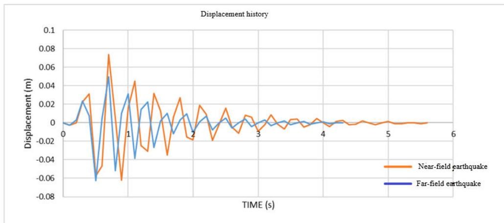
Fig 4. Comparative graph of average response of structure displacement under the near- and far-field earthquake
