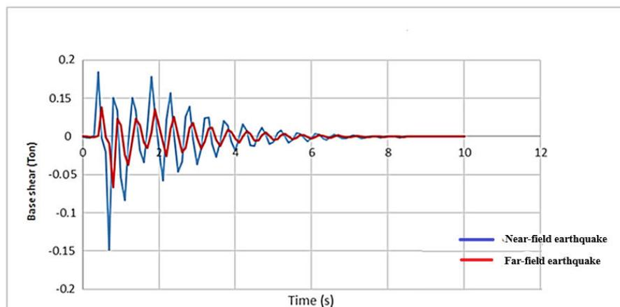
Fig 5. Comparative graph of average response of base shear history under the near- and far-field earthquake
