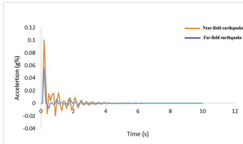
Fig 6. Comparative graph of average response of structure acceleration under the near- and far-field earthquake
